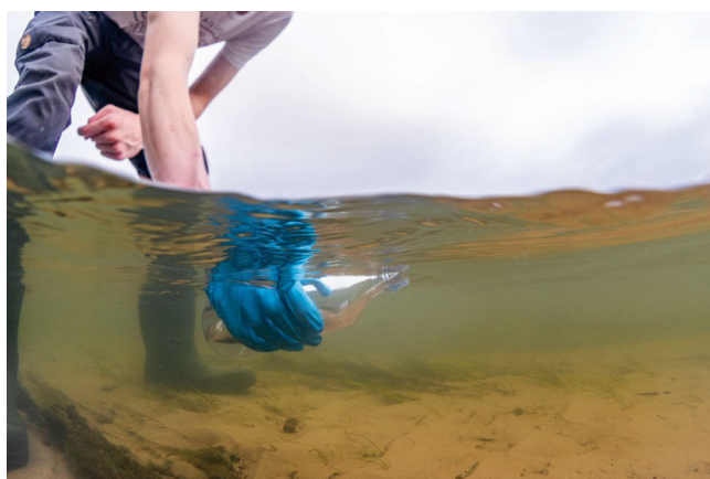
Fig. 3: Water samples for eDNA analyses are collected in sterile bottles
