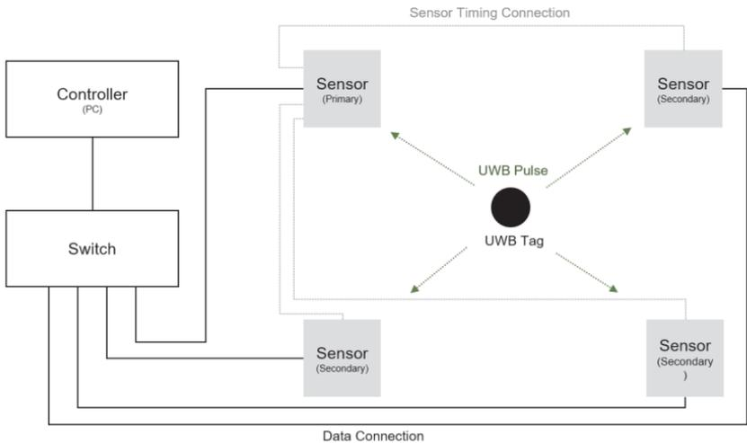
Figure 1: Ubisense architecture (Corrales et al., 2008)
