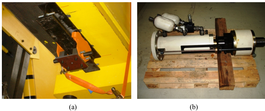
Fig. B.28: Loading setup: a) overhead horizontal traveling support of cyclic actuator, b) cyclic actuator
