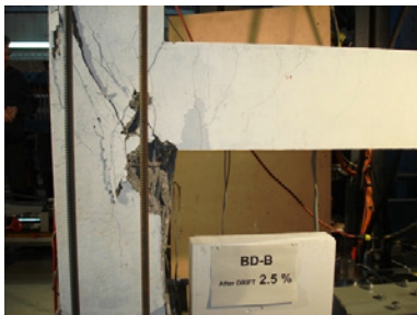
i) Drift 2.5%: Concrete wedges Spall off
