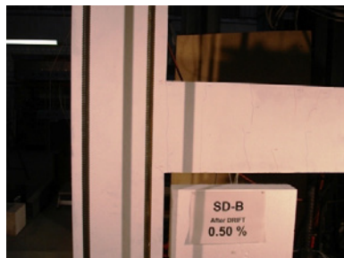
d) Drift 0.5%: First small diagonal cracks at the beam corners of the beam column interface
