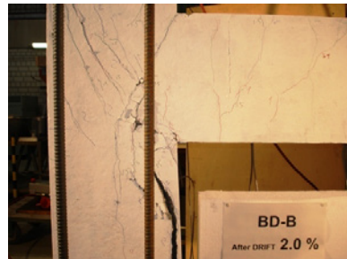
h) Drift 2%: Slippage and pulling-out failure of beam Bot. bars and beginning of concrete spalling
