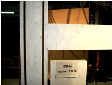
g) Drift 1.5%: First crack in the back of column
