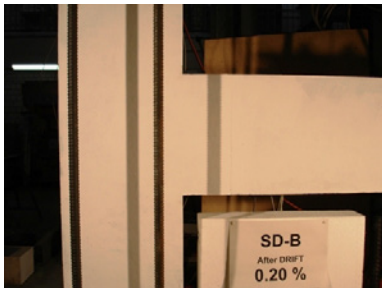
a) Drift 0.2%: No cracks
