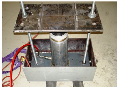
Fig. B.9: Loading setup: Fabricated top compartment
