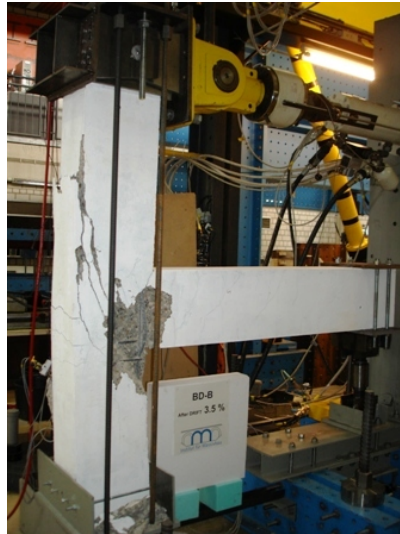
Fig. 4.54: Final failure of specimen BD-B after the first cycle of 3.5% drift
