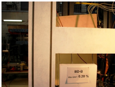
a) Drift 0.20%: No cracks
