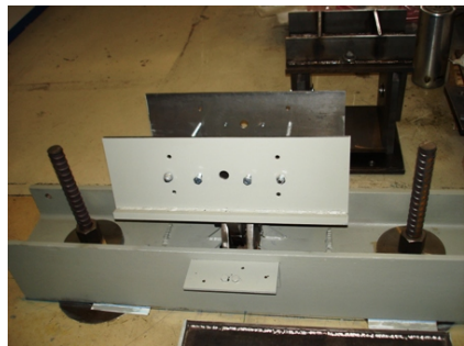
Fig. b.21: Loading setup: Fabrication of fixed support (Det. 5)
