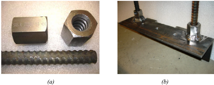
Fig. 4.30: a) SAS 670/800-Stahlwerk Annahütte threaded steel bar with anchor nuts; b) Prepared angle connector (L1) with welded anchor nuts
