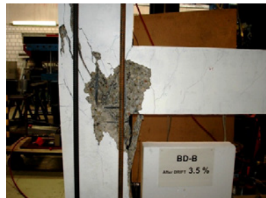
j) Drift 3.5%: Concrete in the joint panel falls down
