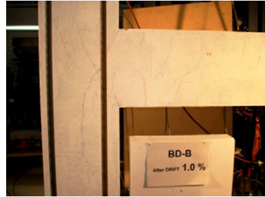
f) Drift 1%: Propagation of the cracks
