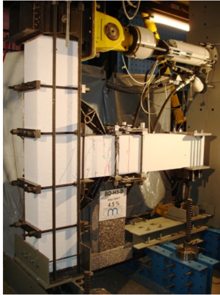
Fig. 4.99: Retrofitted specimen BD-H3-D after 4.5% drifts level
