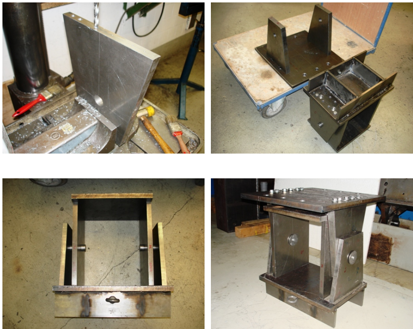
Fig. B.14: Loading setup: Fabrication of second mechanical hinge
