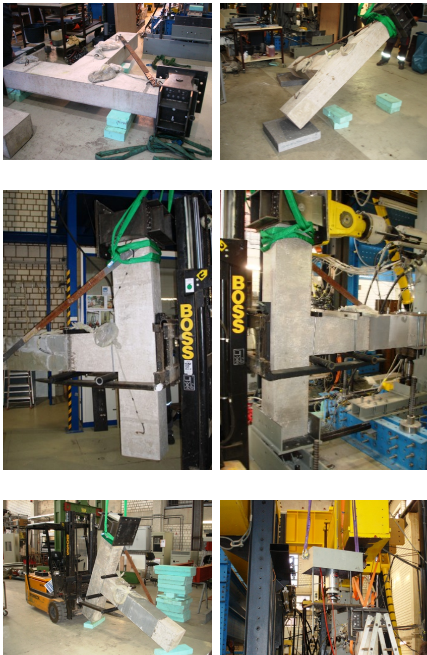
Fig. C.2: Loading setup: Installation of specimens in loading setup
