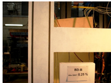
b) Drift 0.25%: Minor hairline cracks in the beam
