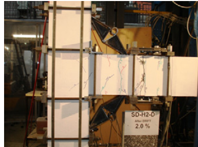
h) Drift 2%: First negative diagonal hairline shear crack of the joint
