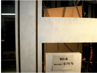
e) Drift 0.75%: First negative diagonal cracking in the joint
