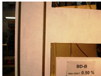
d) Drift 0.50%: First positive diagonal crack in the joint
