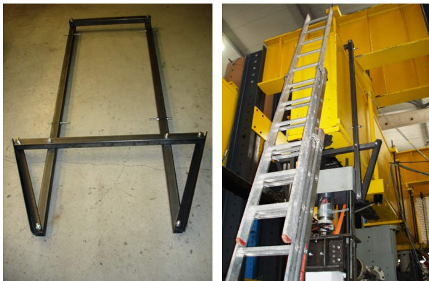
Fig. B.27: Loading setup: fabricated lateral support of test specimens
