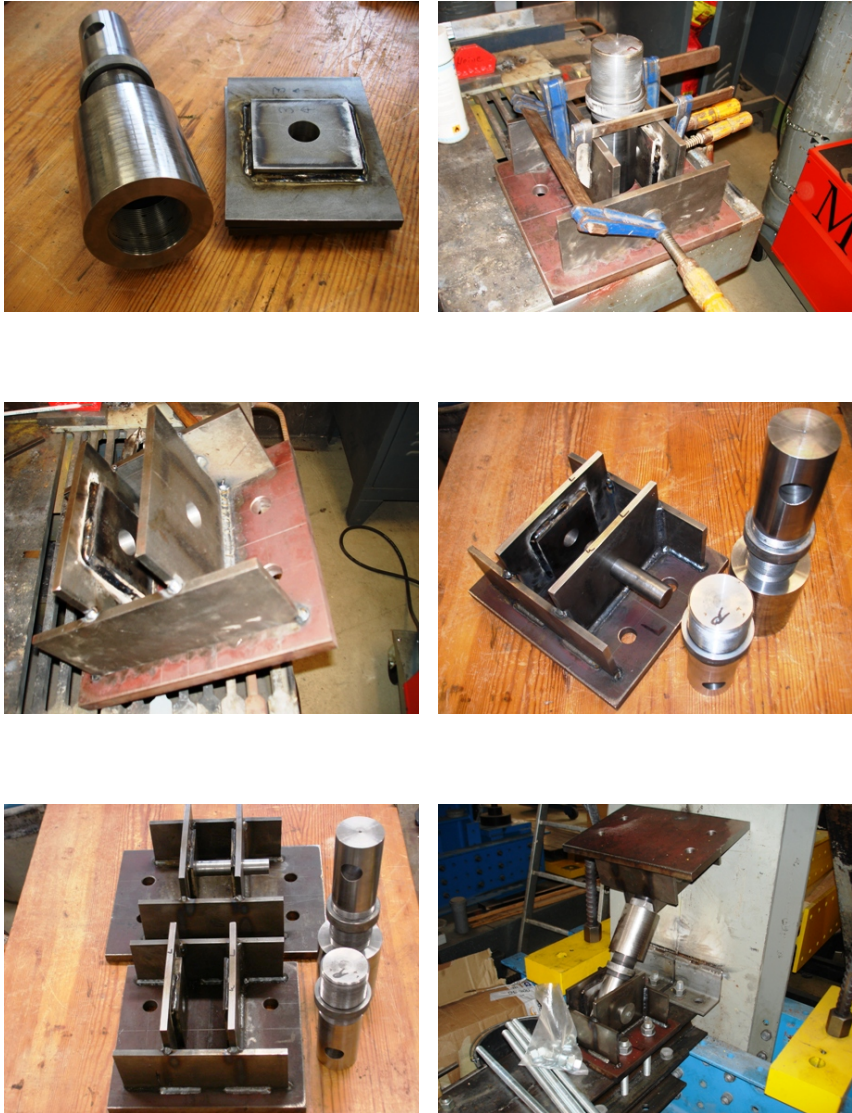
Fig. B.19: Loading setup: Fabrication of movable support (Det. 4)
