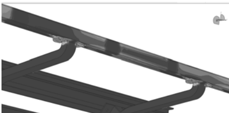
Fig. 10: Von-Mises stress results after a pre-tension load on the bolts
