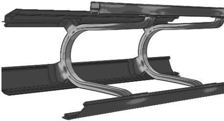
Fig. 13: Von-Mises stress results after applied loads, with maximum E-module value after adding luggage (17000 MPa)
