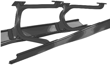
Fig. 20: Frequency response function (FRF) results at 11 Hz with luggage
