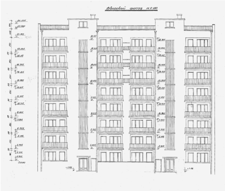
Figure 11: Standard design of an eight-story, two-section, 48-unit residential building, with facade oriented to the yard. Designed by Sh. Kavlashvili (chief architect) and Chachanidze. Source: National Archives of Georgia, Tbilisi
