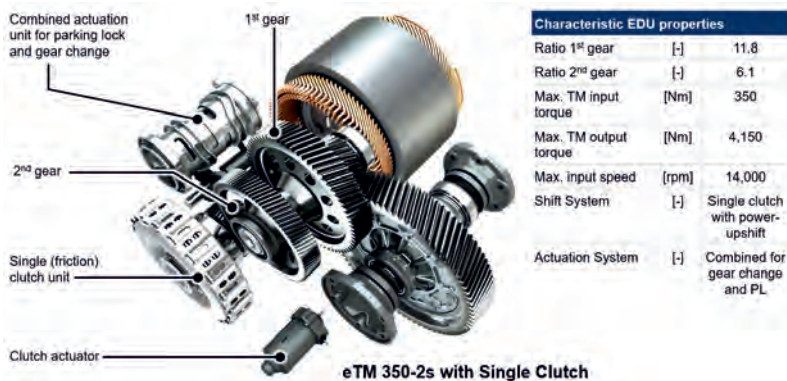
Fig. 10: IAV 2-speed single-clutch transmission design
