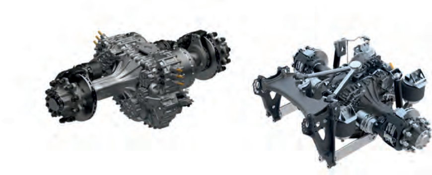
Fig. 1: AVL e-axle with and without suspension system
