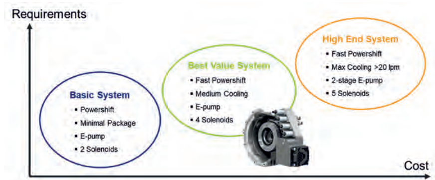
Fig. 11: Potential variants of the target solution
