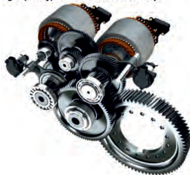
Fig. 15: Digital prototype and core performance data of the new 3-speed E-Drive concept
