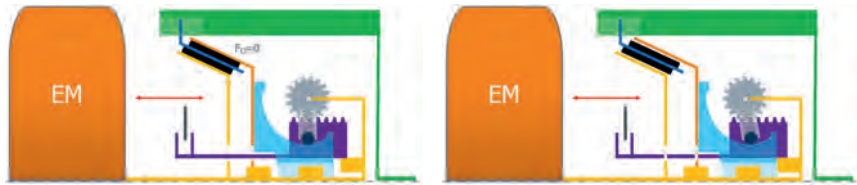
Fig. 8: Diehl ecoClutch FM switching element in intermediate state
