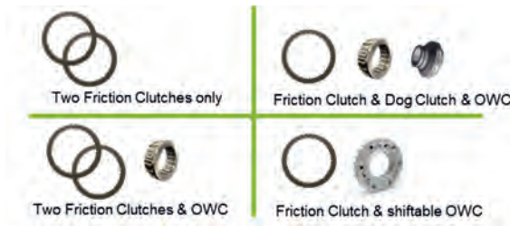
Fig. 5: Shift elements for planetary gear set control
