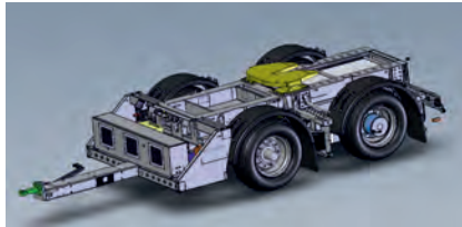
Fig. 7: CAD model of the Smart Power Dolly as designed
