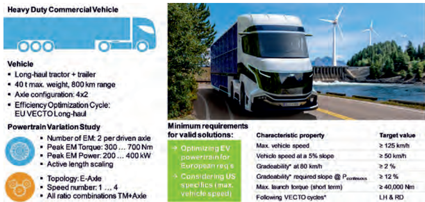
Fig. 10: Boundaries for Powertrain Synthesis study to determine optimized and valid powertrain topologies
