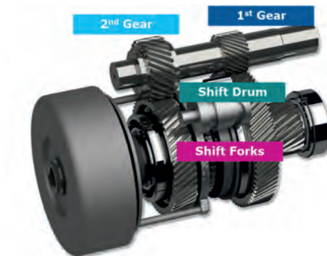
Fig. 6: Transmission gear set and shift concept (© AVL)
