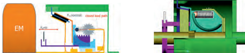
Fig. 7: Diehl ecoClutch FM shifting element in closed state
