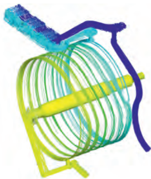
Fig. 1: Streamlines of cooling circuit in an ZF electric axle
