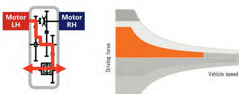
Fig. 3: Torque transmission path of “1-Motor-Low” mode
