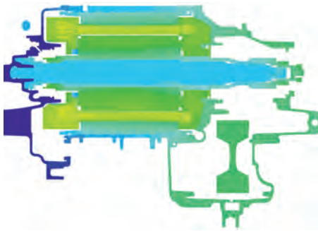
Fig. 2: Temperature distribution in a series production ZF electric axle
