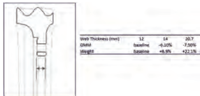
Fig. 10: Modification of web thickness of final gear pair wheel
