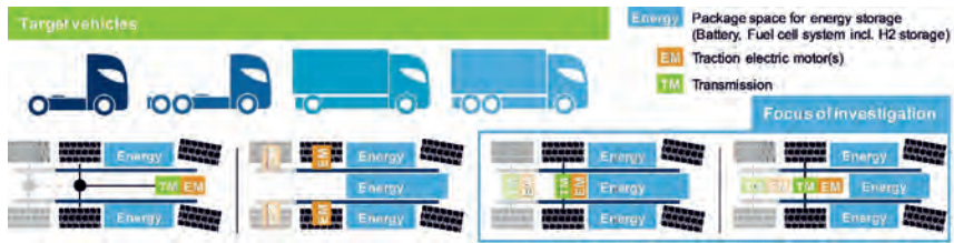
Fig. 7: Powertrain and energy storage installation options in heavy-duty on-road trucks
