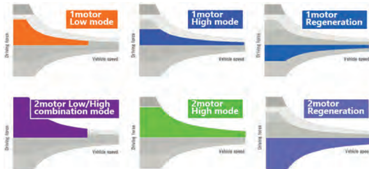
Fig. 2: Torque/speed range of each mode
