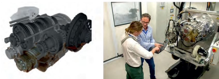
Fig. 2: CFD simulation of lubrication system (left) & physical rig test (right)
