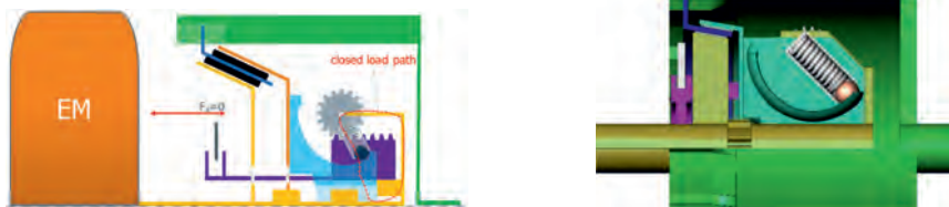
Fig. 9: Diehl ecoClutch FM shifting element in open state
