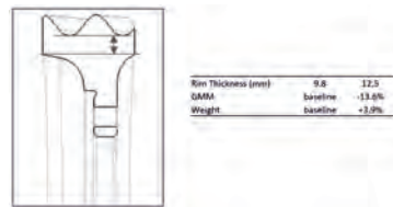
Fig. 11: Modification of rim thickness of final gear pair wheel
