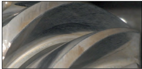
Fig. 1: Running and wear marks on a pinion flank of a hypoid gear
