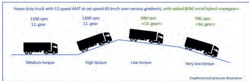
Fig. 5: Illustration of serial hybrid “overdrive” gears.
