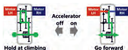
Fig. 10: Hill assist start function
