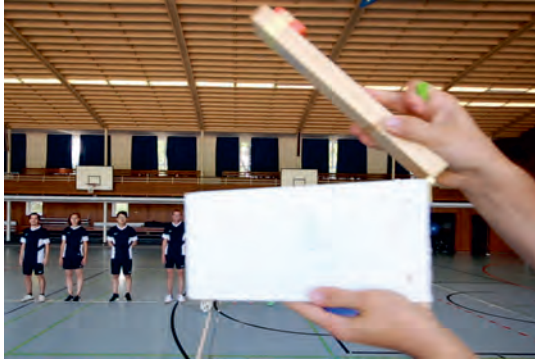
Figure 3.14: Time synchronization using a clapper board.
