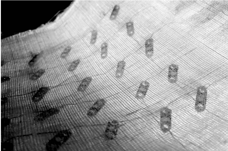
A textile circuit with sewable LED Matrix. 11
