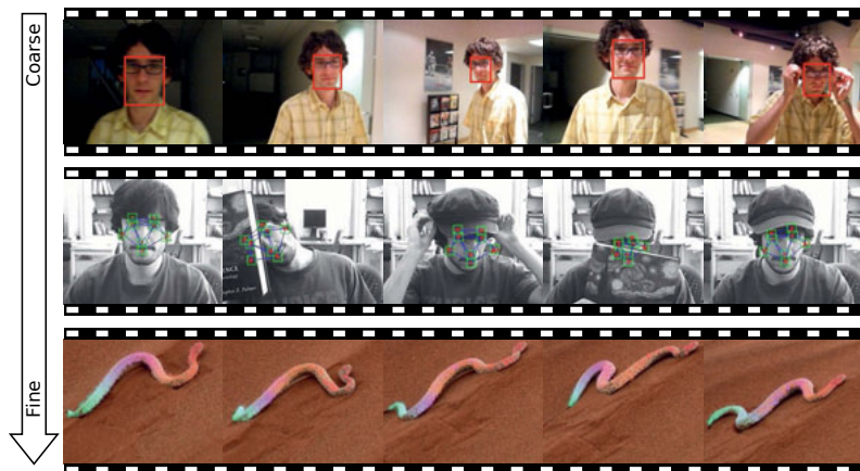
Figure 1.1: Object tracking with varying level of detail. Top: Tracking of the coarse extents of an object (the bounding box, visualized as a red rectangle). Middle: Tracking of an object which is decomposed into smaller parts (green rectangles) which are related to each other (blue lines). Bottom: Fine-scale part-based tracking of articulated objects (parts are color-coded from the head to tail fading from red over blue to green).
