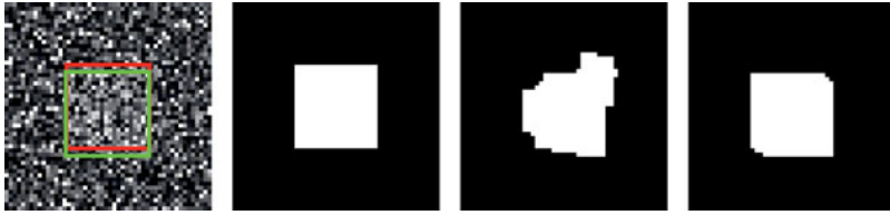
Figure 5.9: Image segmentation with shape prior. Left: Input image corrupted with noise, groundtruth pose (red square), reconstructed pose (green square). Middle left: Groundtruth segmentation. Middle right: Graph cut segmentation. Right: Our approach.
