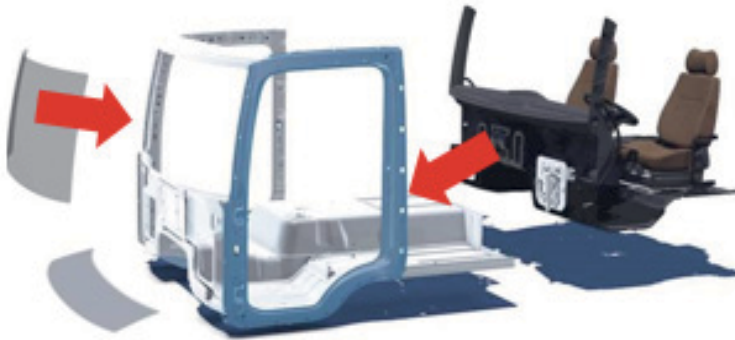
Fig. 3: Pre-assembled cabin platform module
