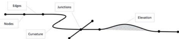
Fig. 14: Example of a virtual road network
