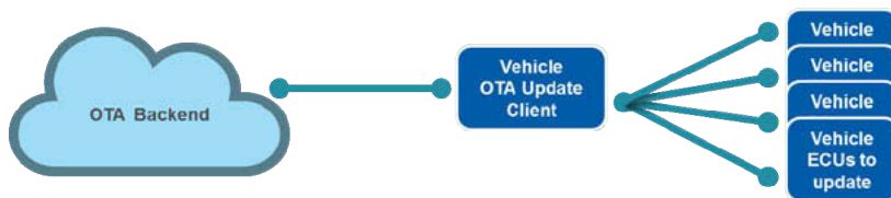
Fig. 1: The three major components of an Over The Air software update solution
