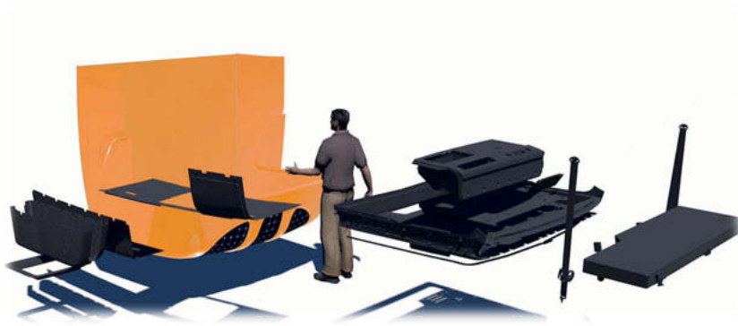
Fig. 6: Ergonomic pre-assembly of cap module
