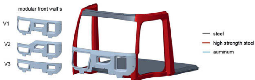
Fig. 2: Design & material concept of cabin platform
