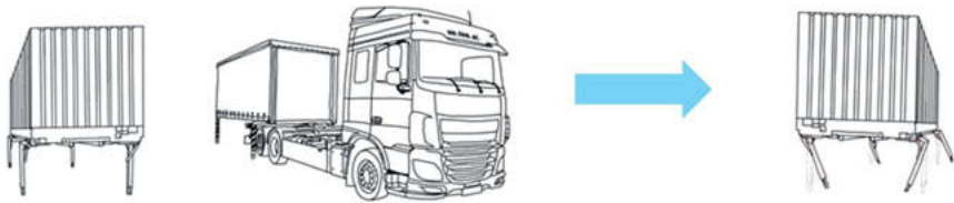
Fig. 2: Maneuvering errors often lead to expensive damage of the swap body as well as to the vehicle and depot infrastructure.
