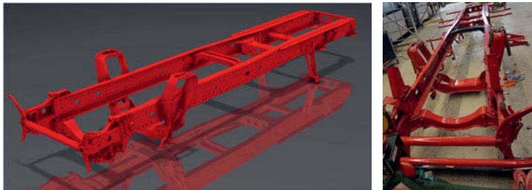
Reference vehicle ladder-type frame (photos from the vehicle dismantling)
