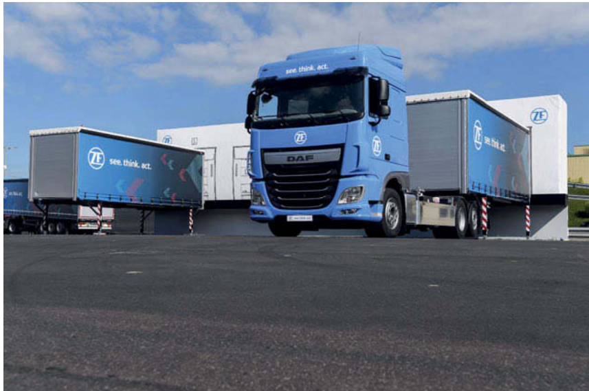
Fig. 1: The ZF Innovation Truck: Fitted with Swap Body Assistance, it autonomously masters lifting, shifting and stacking at depots and other premises.
