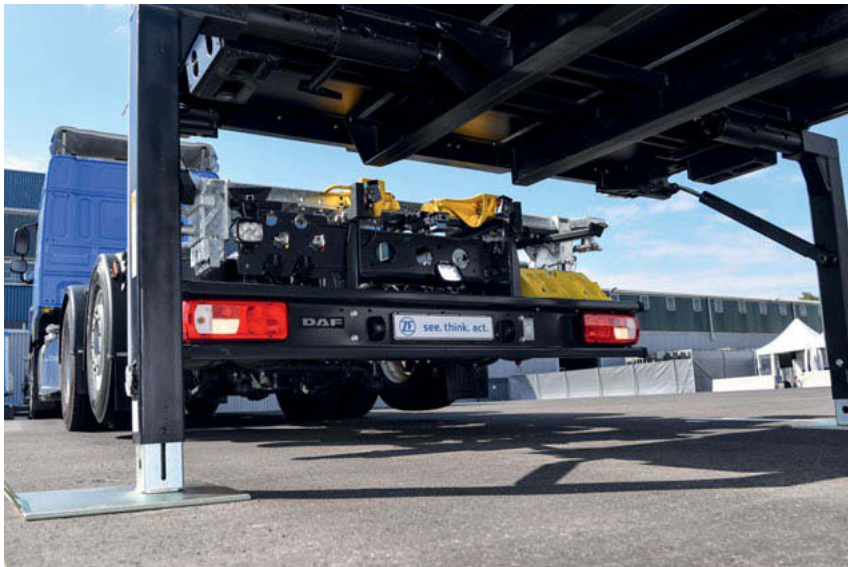
Fig. 9: The combination of sensor set, actuators, high-performance computer and intelligent algorithms enable the precise, autonomous driving of the truck under the swap body with high precision.
