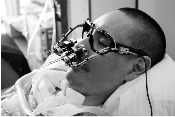
2.16: Tempt1 wearing his eye-tracking device; Source: The EyeWriter Project.
