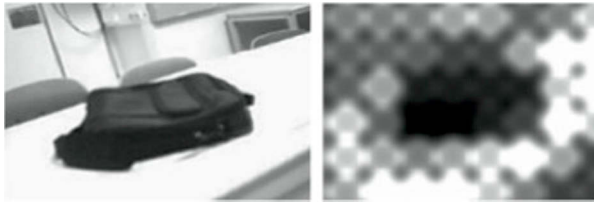
2.17: Simulation of visual perception through a retina implant; Source: Hornig & Velikay-Parel 2013: 473.
