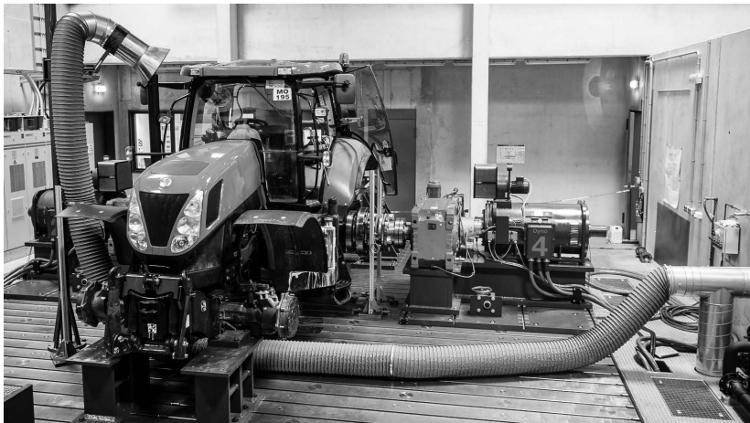
Fig. 2: Tractor Test Bench: Setup of the automatic calibration of the real tractor
