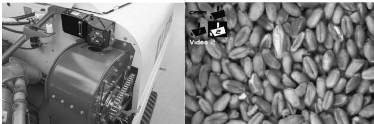
Fig. 3: Position of the GRAIN QUALITY CAMERA and an evaluated picture
