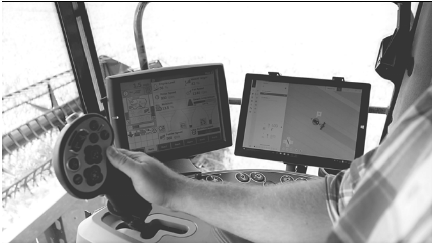
Fig. 3: On-board command and control system concept shown as part of CNH Industrial Autonomous Concept Vehicle launch at Farm Progress Show in Boone, IA, USA in August 2016.
