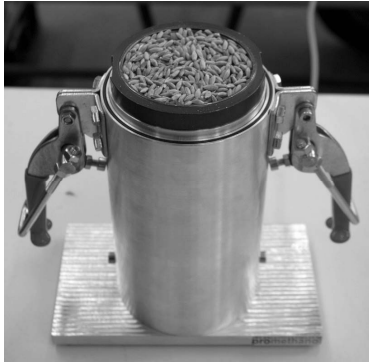
Fig. 1: Lower part of the chondrometre inside the air pycnometre.
