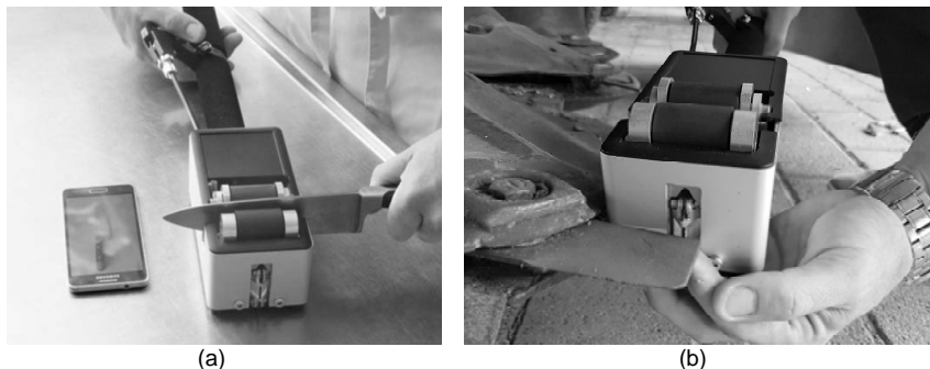
Fig. 4: Roller infeed application for investigating a kitchen knife (a) and front end application for investigating a mower knife (b)
