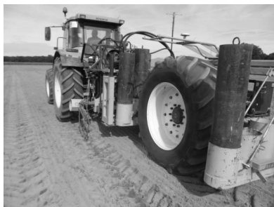
Fig. 2: IRSTEA single wheel tester performing a tire efficiency test in a field
