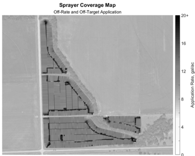
Fig. 3: High resolution as-applied coverage map of Field 3 generated by the PACT program.
