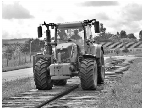
Fig. 3: Test drive with instrumented test tractor on ISO 5008 smoother track
