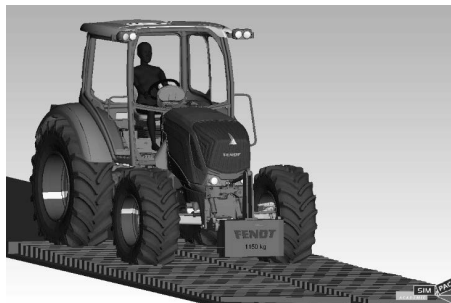
Fig. 1: Multi-body simulation model of the Fendt 313 Vario test tractor on ISO 5008 smoother track standard roadway
