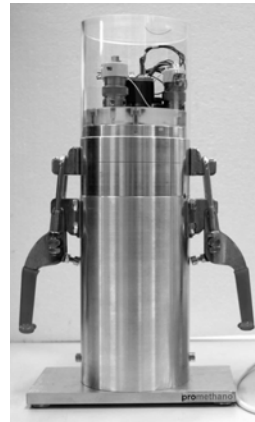
Fig. 2: Air pycnometre, closed airtight.
