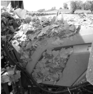
Fig. 2: Plant residues at the fan grill while trimming vineyards
