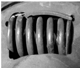
Figure 5: Dramatic wear of compression springs and any wear. The situation in the DMF was fundamentally different. Isolation was present here over the entire speed range and the damper springs were required to compensate vibration at each engine ignition.
