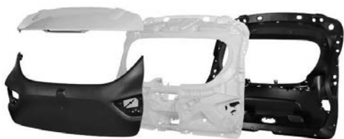
Fig. 6: The three-part construction that forms the Clio's lift-gate
