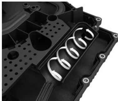
Fig. 4: Centrifugal separation in the media lines carrier to separate the air-oil mixture
