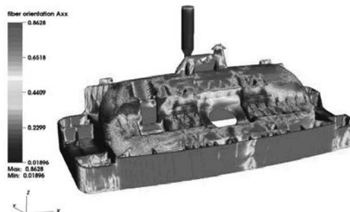
Fig. 17: A_{xx} component of the fiber-orientation tensor following filling of the airbag housing.
