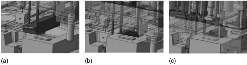
Fig. 11: Selected stages of the closing process: (a) entry of the split into the lower mold cavity, (b) definition of the core block in the lower mold, (c) mold fully closed
