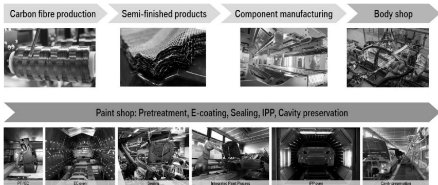
Fig. 4: Process chain for hot-curing adhesives in the Carbon Core production concept [4]
