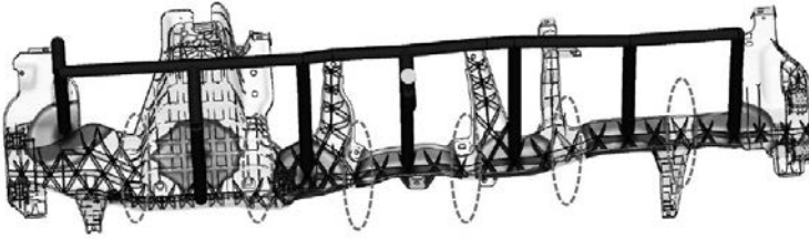
Fig. 5: Emergence of major weld lines - 40% mold filling
