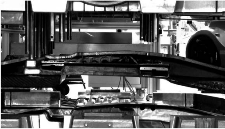
Fig. 9: Undercuts mean that the component must be demolded laterally
