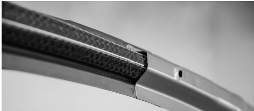
Fig. 9: RTM braided component, roof frame reinforcement
