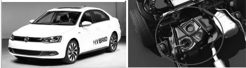
Fig. 9: The US model VW Jetta Hybrid and installation location of the hybrid plastic tank (source: VW)
