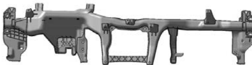
Fig. 4: Variant 2 - organic sheet in transverse combination and back-injected with thermoplastic material
