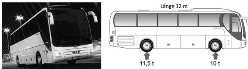
Fig. 1: The MAN Lion's Coach tour bus in operation and the axle load distribution of a two-axle bus
