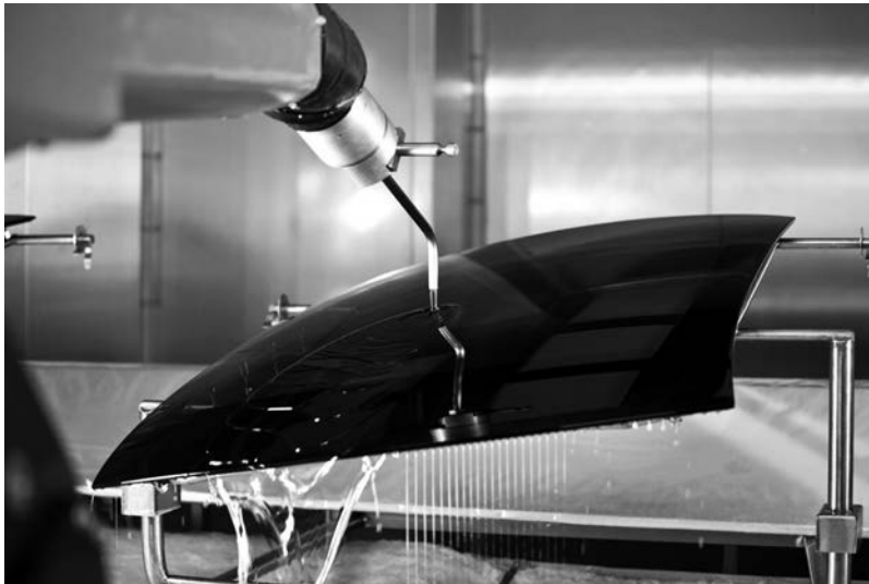
Fig. 3: Coating a polycarbonate element by flooding
