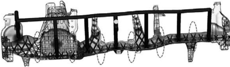
Fig. 6: Main weld lines closed at the surface, further flushing due to incomplete mold filling → weld lines are shifted in the core.
