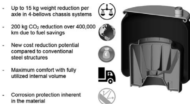
Fig. 8: Benefits of air springs with a plastic piston
