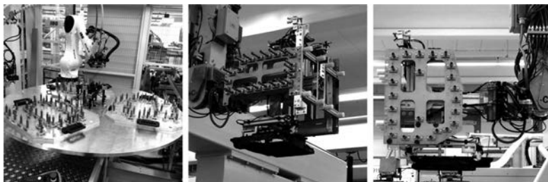
Fig. 10: Left: Rotary indexing table for the bushings; center and right: placement and removal handling units on the nozzle and ejector sides respectively.
