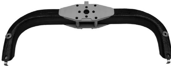
Fig. 5: CFRP / steel hybrid air spring carrier
