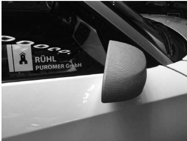
Fig. 6: Components with a sharkskin surface in the interior and exterior as a demonstrator at the SPE Award Ceremony 2015
