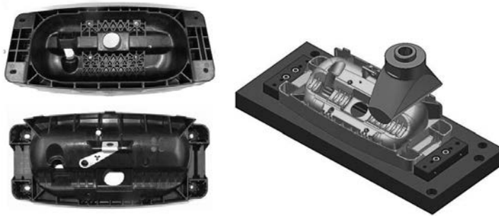
Fig. 16: Airbag housing showing exterior (top left) and interior (bottom left) as well as the construction developed for the clamping device for component testing, showing the clamped component and the drop-weight tower punch.
