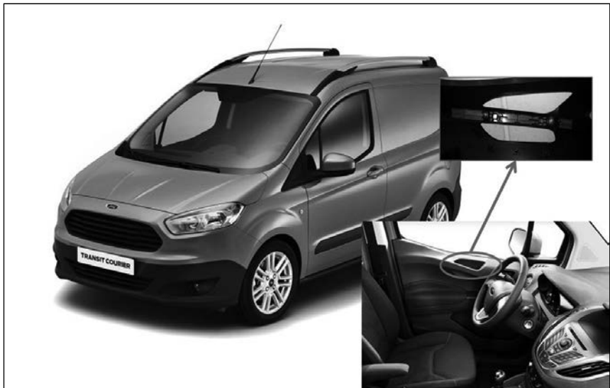
Fig. 8: 'Local reinforcement' in the door trim of the Ford Transit Courier B460 (source: Ford Motor Company)
