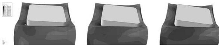
Fig. 12: The equilibrium position of the rigid mass experiencing 0.1 g (left), 0.2 g (right) and 0.3 g (right) lateral accelerations
