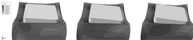
Fig. 12: The equilibrium position of the rigid mass experiencing 0.1 g (left), 0.2 g (right) and 0.3 g (right) lateral accelerations
