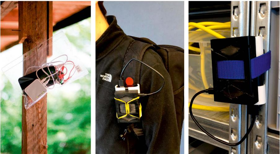
**Fig. 1** The technical artifact is made up of a RaspberryPi, an SD card and battery. Different casings and ways of attaching it to places have been experimented with throughout the various use cases. The solutions depicted here highlight the versatility and portability of the toolkit. Design Research Lab.
