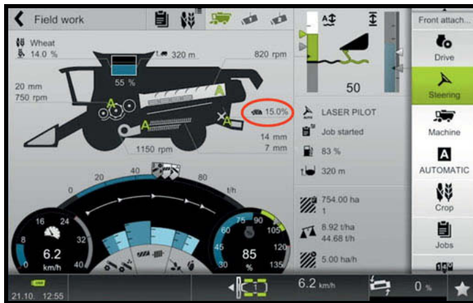
Fig. 5: Visualisation of the straw moisture value on the machine control terminal
