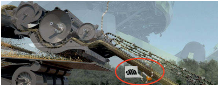
Fig. 3: Sensor position underneath the feeder house at the front of the machine
