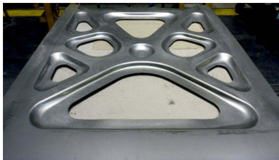
Fig. 6: Formed sheet metal part using rubber pad forming
