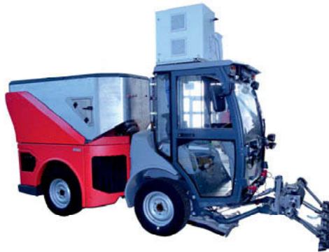
Fig. 3: Cutter bar, control and test equipment mounted on implement carrier
