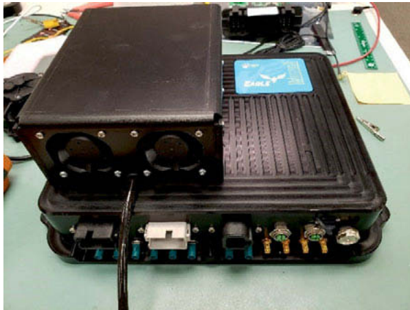
Fig. 6: JCA Eagle - Ruggedized Advanced Processing Platform for Autonomous Systems
