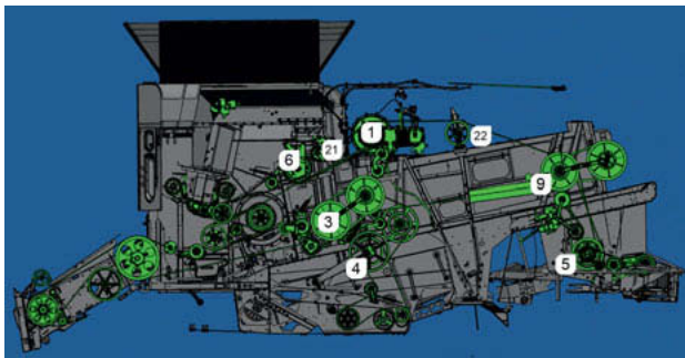
Fig. 4: Driveline left hand side of new generation combine (twin rotor)
