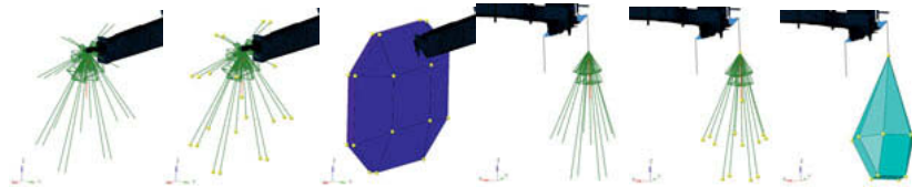
Fig. 2: Dynamic ranges of interaction forces on boundary nodes. The displayed polyhedra in force space are formed by maximum force events (green arrows) that can be calculated according to [4]. Red arrows: static reaction forces.
