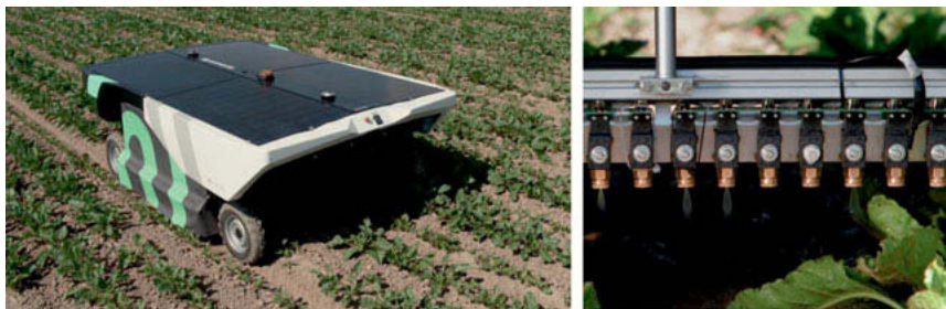
Fig. 4: Second design in operation in sugar beet (left), high nozzle density spray bar (right).
