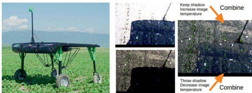
Fig. 3: Robot at work in sugar beet (left), dual exposure and image combination to remove machine shadow and increase image SNR and plant identification rate.
