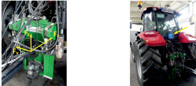
Fig. 1: Device to measuring the forces between tractor and trailer (left image) and location of the IMU-box behind the tractor cabin (right image)
