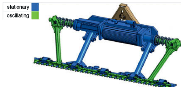
Fig. 2: Detailed prototype concept for the electric direct drive bar mower
