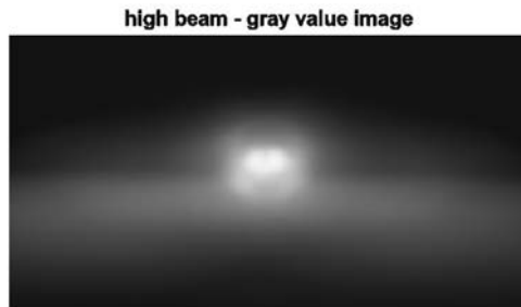
Fig. 4: Image of the modeled high beam of a Porsche PDLs+ LED headlamp
