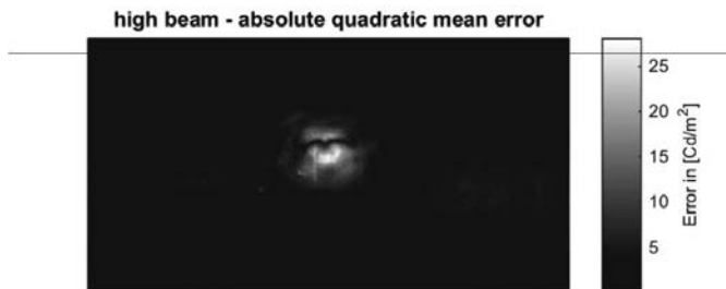
Fig. 5: Absolute quadratic mean error between modeled and real high beam distribution
