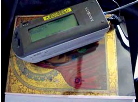
Figure 8.3. Minolta CM-2600d measuring reflectance spectra on selected areas of the Russian icon.
