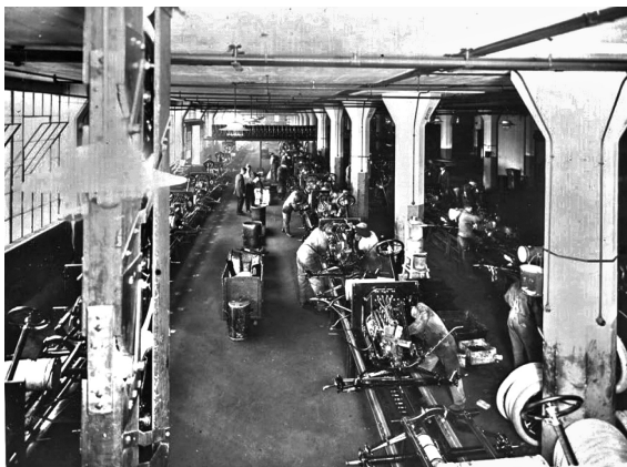
Abbildung 13: Chassis-Montagelinie in Highland Park (1914)
