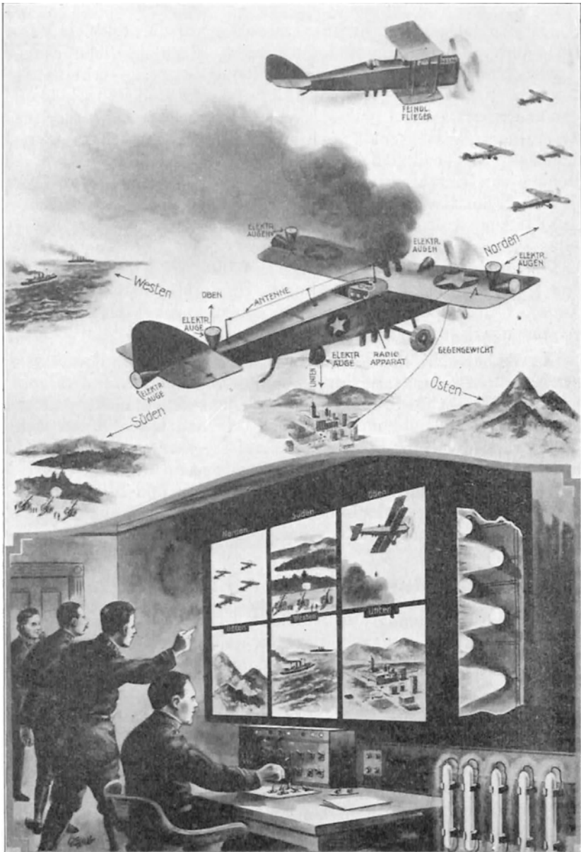
Figure 9: Drawing that appeared in Fernbildtechnik und elektrisches Fernsehen by Peter Lertes (1926), an engineer from Leipzig. The airplane has “elktr. Augen” in all directions which correspond with the monitors in the console below. Like figure 4 (bottom left) the artist has ‘cut open’ the hardware to show what is inside.
