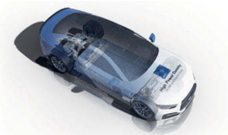
Fig. 12: High Speed E-Axis Integrated in Vehicle14
