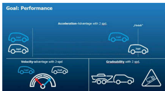
Fig. 2: Performance can be enhanced with a 2-speed gearbox.
