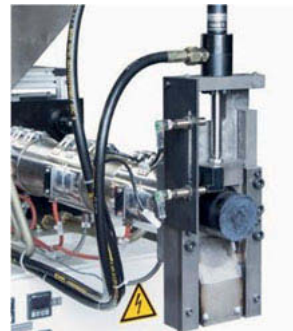
Fig. 3: Screw pre-plastification unit [2]
