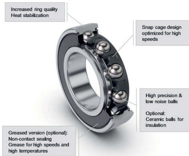
Fig. 2: HSMB 1.3 bearing with characteristics
