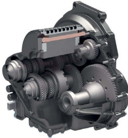
Fig. 8: XT20 DHT 3D Model with a 50 kW EM
