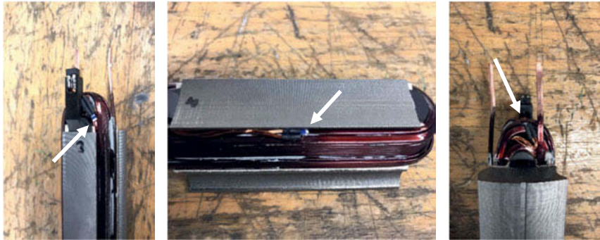
Fig. 20: Placement of the temperature sensors prior to gluing
