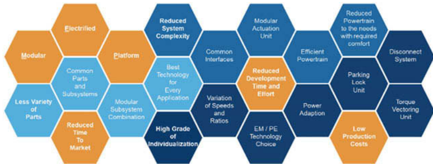
Fig. 9: Creation of a modular drivetrain platform for electrified passenger cars
