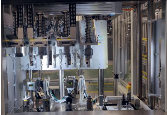
Fig. 25: Pressing machine for bearings installation.
