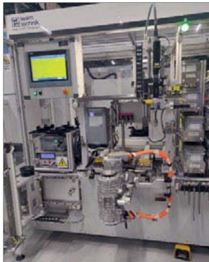
Fig. 32: Leakage test machine (oil and water circuits) and electric insulation machine
