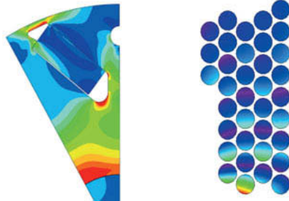
Fig. 2 left: Mechanical Simulation (von Mises stress) at 36000 rpm, Right: Current Density in the Conductors of One Slot at Maximum Rotation Speed
