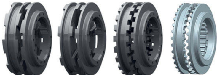
Fig. 5: Dog clutches of Speed2E (dark grey [2]) and Speed4E (light grey)
