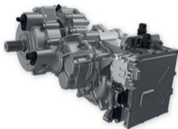
Fig 9: 48V 25kW eDRIVE specification
