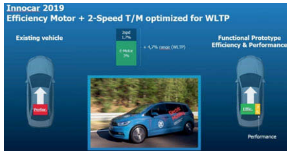
Fig. 6: Demonstration vehicle of ZF: by replacing a single speed drive by a 2-speed drive, 4,7% range extension could be achieved. [1]
