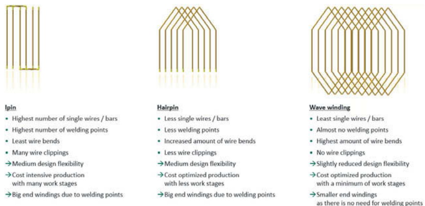
Fig. 8: Excerpt of possible stator bar wound winding technologies
