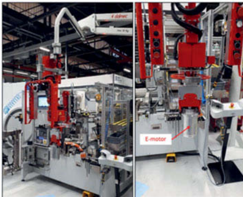
Fig. 30: Dalmec system for e-machine handling
