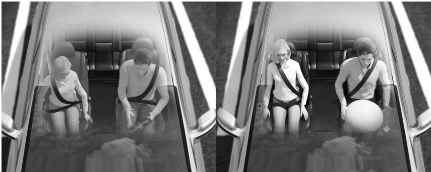
Fig. 5: During a crash objects need to be moved away from occupants
