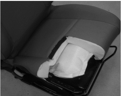
Fig 3b: Pelvis restraint cushion installation
