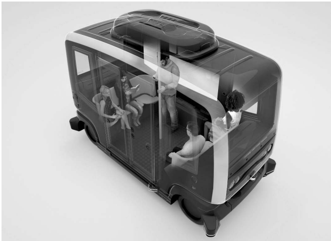
Fig. 4: AD vehicle of the People Mover type as shown by Continental at the Frankfurt Motor Show 2017; note the mix of undefined bench seat positions and standing capacity
