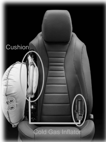
Fig. 2: Schematic view of PRE-SAFE® Impulse Side main components
