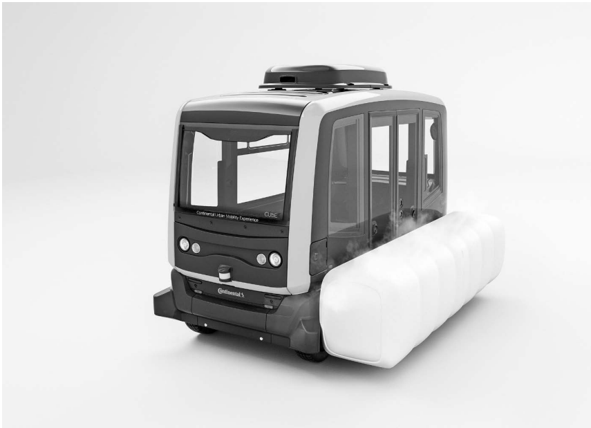
Fig. 10: Outside airbags can help to compensate the lack of crumple zones in electrified vehicles
