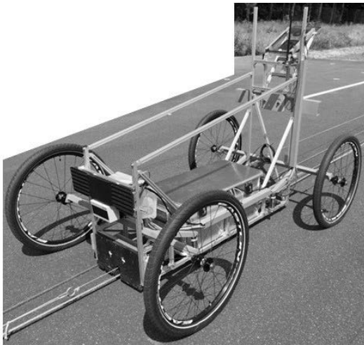
Fig. 8: The sensor cart represents a vehicle front end with geometrically correct sensor array
