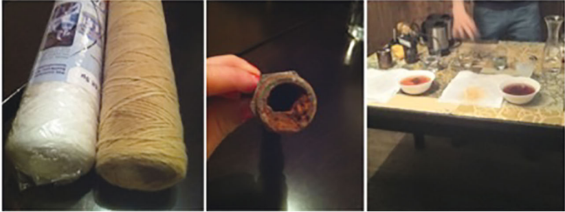
Figure 3: A new and a used cotton filter, the rusty inside of a drinking water pipe and an experimental setting with a bowl of tea made with filtered water (left) and one with unfiltered tap water (right).
