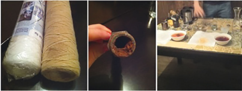
Figure 3: A new and a used cotton filter, the rusty inside of a drinking water pipe and an experimental setting with a bowl of tea made with filtered water (left) and one with unfiltered tap water (right).
