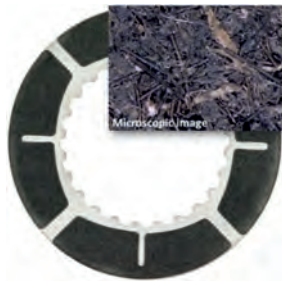
Fig. 7: MC 650 on a disc for a rear axle differential including a microscopic image illustrating the high amount of carbon fibers in the material matrix.
