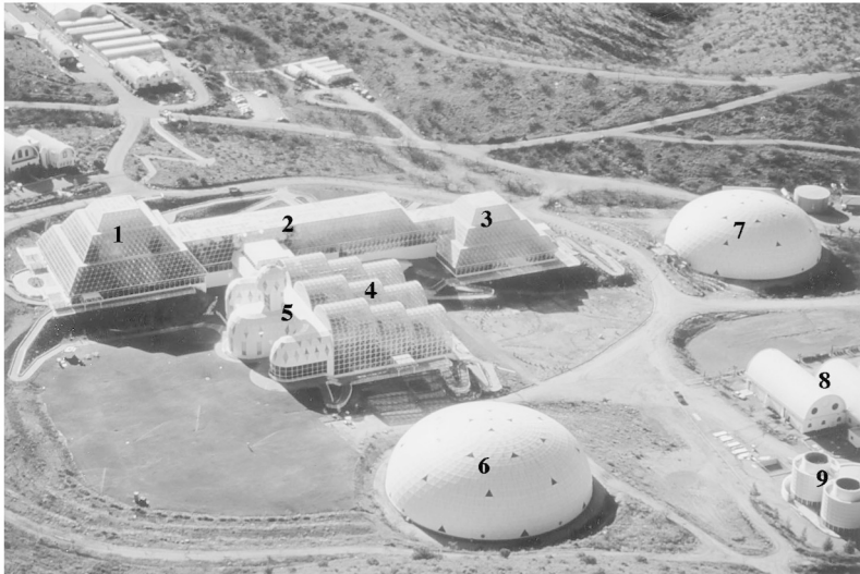
Fig. 1. Aerial view of Biosphere 2 facing southeast showing locations of: 1, rainforest; 2, savannah/ocean/marsh; 3, desert; 4, intensive agriculture; 5, habitat; 6, west lung; 7, south lung; 8, energy center; and 9, cooling towers.
