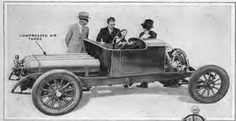
A side view of the compressed air car, showing the four fuel tanks which will drive the car 500 miles at a speed of 35 miles an hour. The engine requires no cooling system, no ignition system, no carburetor, nor the hundreds of moving parts included in a standard gasoline motor.
