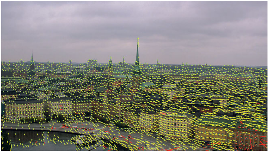
(c) OldTownCross, manual labeling. The tracking fails in some parts (bottom right, red lines) due to repetitive structure (windows). Moreover, the individual movement of the waves on the sea (bottom left) makes the manual and automatic classification difficult. Displacement vectors of the background are colored yellow, outliers and moving objects are colored red.
