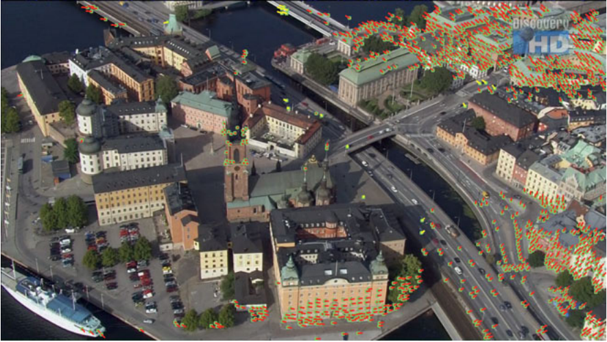
(a) Stockholm, homography classifier. Upper right and bottom regions are marked as moving due to the homography plane not being fitted onto the ground plane (mostly false positives).
