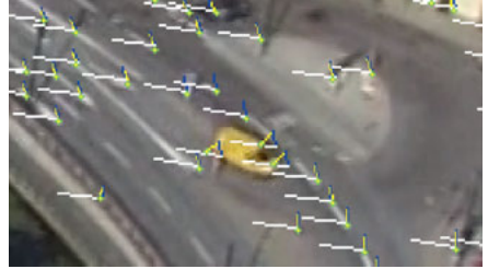
(b) Stockholm, motion parallax predictor classifier. Slow vehicles are not detected if they move along the predicted epipolar line segment (green cross close to the white line at the yellow van).
