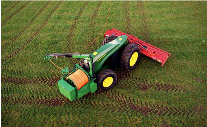
Fig. 2: Autonomous GridCON tractor with electrically driven implement
