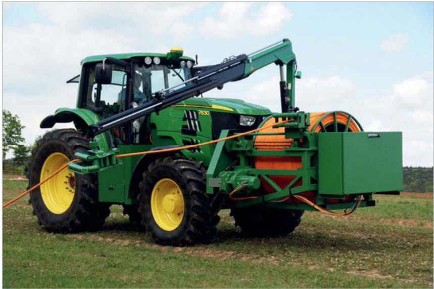
Fig. 1: Battery-electric tractor with permanent connection to the electric power grid
