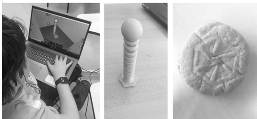
Figure 3: Ricsi, an 8th-grade student, is preparing a cookie stamp for the lower-grade students' activity, designed with the school logo in Tinkercad and independently prepared for 3D printing. Based on his own idea, the tool has several handle versions to ensure that children with different abilities can confidently grip the tool.
