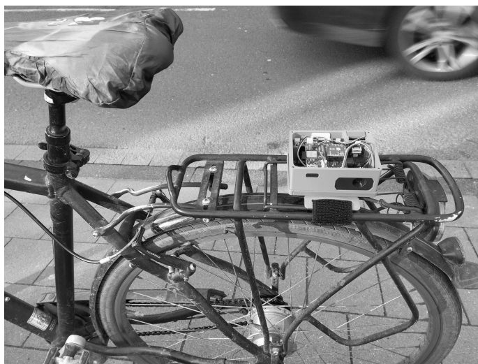
Figure 3. Sensor (in black) in a 3D printed case together with the senseBox MCU S2 on a bicycle. The sensor is oriented to the left side of the bicycle.
