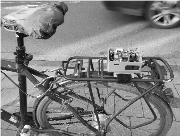
Figure 3. Sensor (in black) in a 3D printed case together with the senseBox MCU S2 on a bicycle. The sensor is oriented to the left side of the bicycle.
