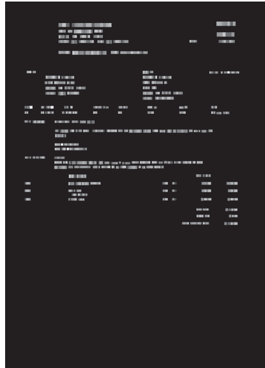
Figure 2: Image of a document page (left) and its character grid (Chargrid) representation (right). Each pixel overlapping with the bounding box location of a character on the document page is mapped to the vocabulary index of that character. The Chargrid representation incorporates textual as well as layout information such as text position and font size.
