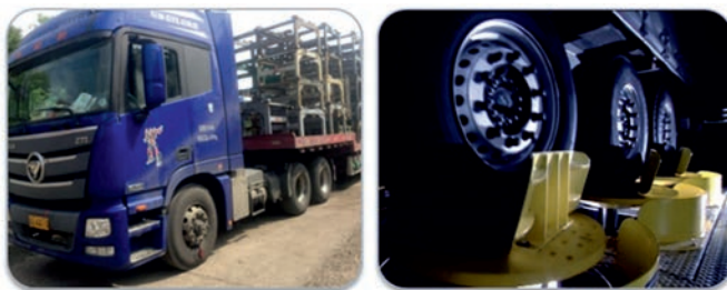
Fig. 7: left: Recording of load spectra for demanding operating conditions, right: Vehicle test bench operated with measured road load spectra.
