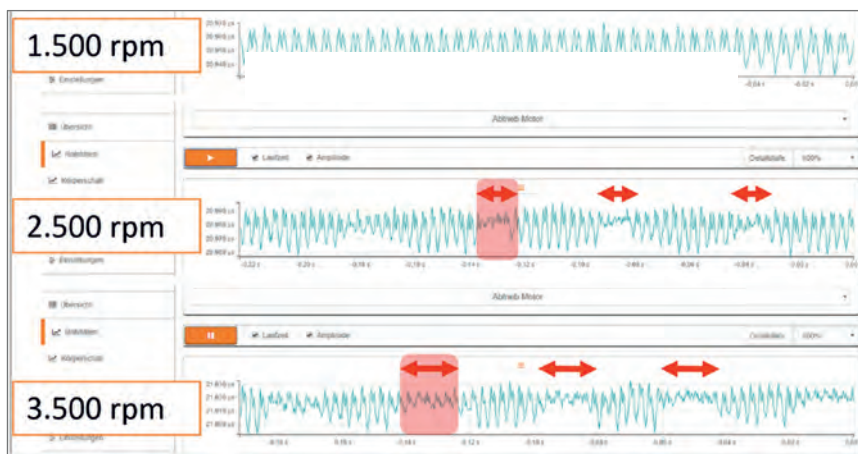
Fig. 5: Screenshot of the BeMoS Web-APP showing the "fingerprints" of the rolling elements in the SAW-time measurement signal for three different shaft speeds with maximum oil filling and counterclockwise rotation
