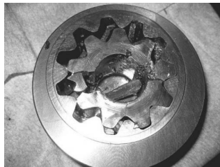
Fig. 22: Damaged gearbox oil pump (9 teeth).
