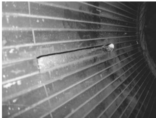
Fig. 6: Missing part of the generator stator bar as photographed during the asset inspection.
