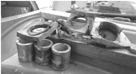
Fig. 12: Damaged anti-vibration mount on the generator.
