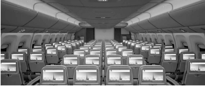
Figure 5.1: Array of screens 'carved out' of the seat-backs on an Emirates Boeing 777.
