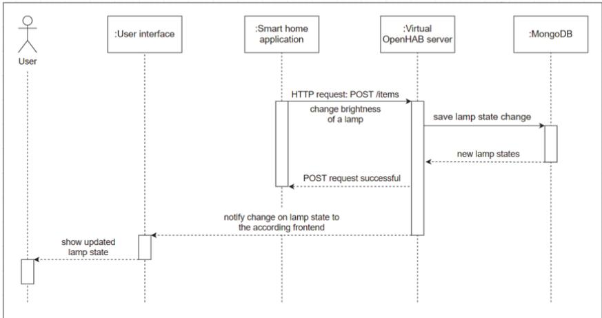
Figure 3. Sequence diagram of a typical scenario
