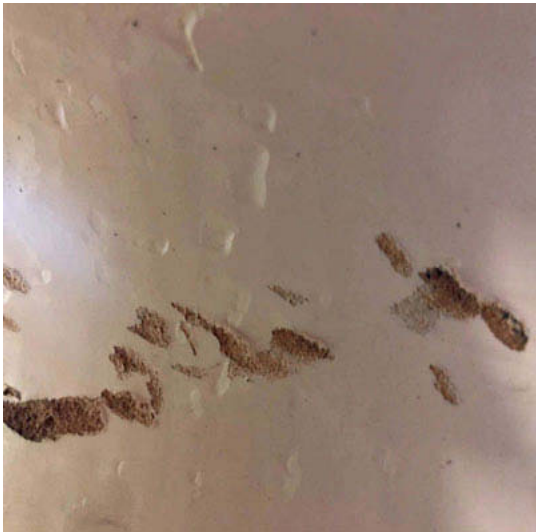
Photo 1. Inside layer of hose showed next to typical erosion marks also strange crater like damages
