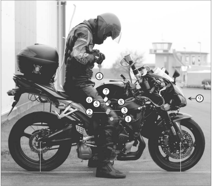
Figure 4.13: Overview of the ready BSTAM Prototype Motorcycle (PMC) Setup with different center of gravity locations
