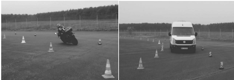
Figure 5.1: Top: Overview of August Euler Airfield proving ground with two different test locations (1: R50, 2: R70). Bottom: Typical positioning of the test motorcycle and a transporter (as a reference for lane width) within the lane at location (1, R50)
