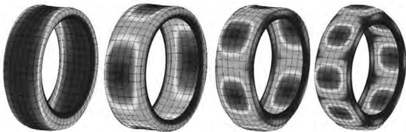
Fig. 5: Radial tire modes (1,0) , (2,0) , (3,0) , (4,0) of non-deflected, non-rotating tire
