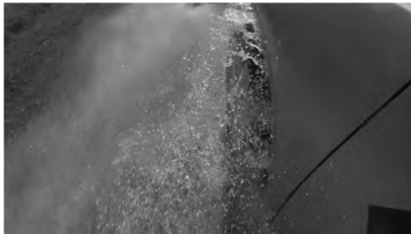
Fig. 3: Characteristic splash water situation in an aquaplaning critical situation
