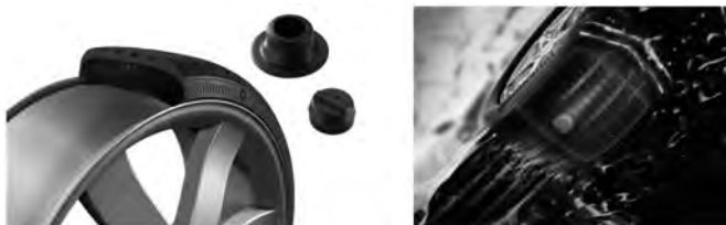
Fig. 4: eTIS sensor with container and tire cross section (left). eTIS Sensor in the innerliner with footprint region treading water (right).
