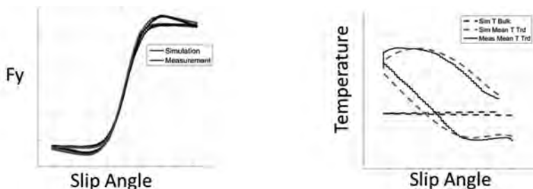
Fig. 7: Validation of thermo-mechanical model for typical sweep experiment
