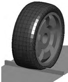
Fig. 9: Schematic setup of a cleat run experiment
