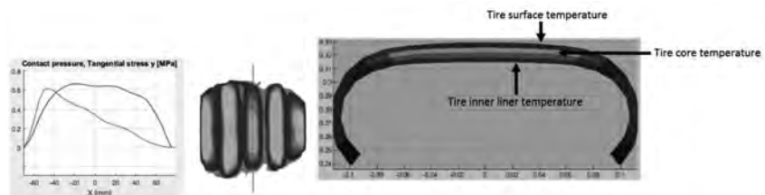
Fig. 13: Contact patch local pressure distribution (left) at 1° slip angle (blue: normal pressure, red: tangential stress) for the central rib and corresponding distribution (right) of the temperature in the tire cross section.
