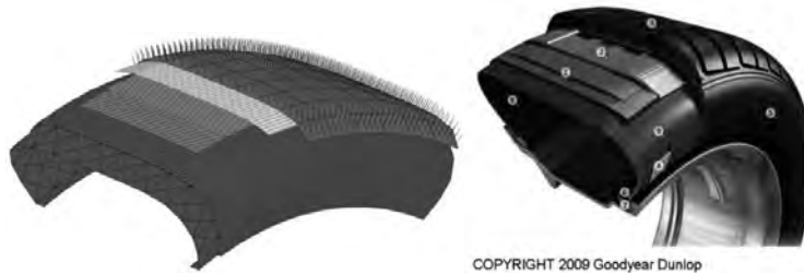
Fig. 2: Functional component layers of the tire
