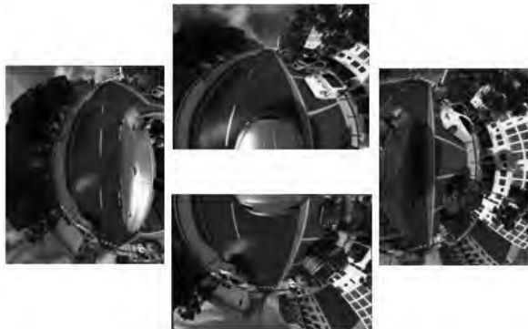
Fig. 2: All four surround view single images with fisheye optics for vehicle near field sensing
