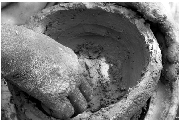
Fig. 15: After a cursory drawing of the rings the potter fills the bottom of the rough-out. This is done by crushing a lump of clay and careful smoothing of the bottom belly junction. Further coils are then superimposed to rough-out the rest of the upper part of the vessel.
