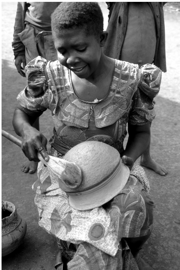
Fig. 6: Once the vessel is shaped and decorated, the potter cuts the outer junction between belly and bottom and beats the external surface with a wooden paddle (Photo: P. Petit).
