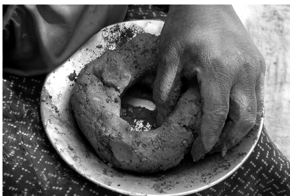
Fig. 12: A ring is shaped from a lump and laid on an enamel support (LUB.01, Luba potter, Lubumbashi).
