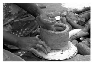
Fig. 3: The coil junctions are smoothed by drawing the clay downwards with the thumb (NKO.01, Luba potter, Nkulu Ma-
