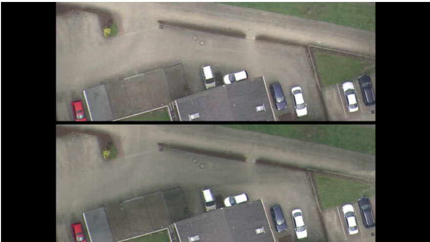
(b) 350 m sequence, best quality (top: reference, 5282 kbit/s; bottom: ROI coding, 5131 kbit/s)
