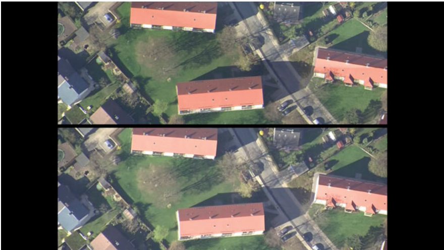
(f) 1000 m sequence, best quality (top: ROI coding, 5156 kbit/s; bottom: reference, 5243 kbit/s)
