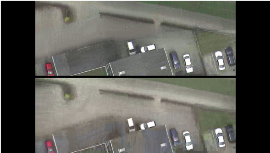
(a) 350 m sequence, worst quality (top: ROI coding, 117 kbit/s; bottom: reference, 126 kbit/s)
