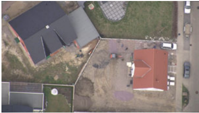
(a) 350 m sequence, ground resolution: 43 \frac{\text{pel}}{\text{m}}
