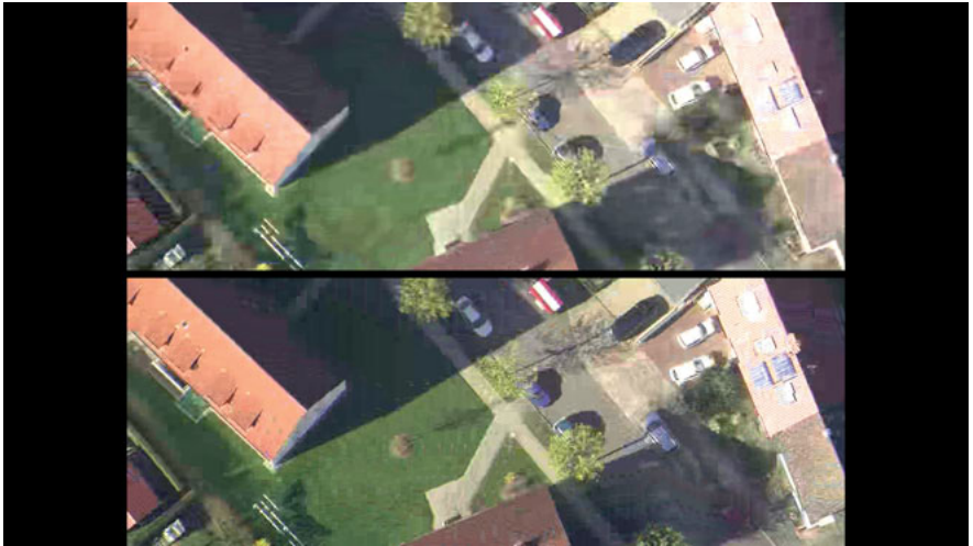
(c) 500 m sequence, worst quality (top: reference, 138 kbit/s; bottom: ROI coding, 126 kbit/s)
