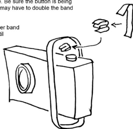
You can add a second loop or a rubber band and hook it on the bottom of the bottle to hold the camera firmly against the top.
