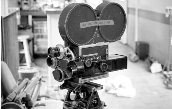
Fig. 83: A Bell & Howell 2709 35 mm movie camera from 1922 with a double-compartment film magazine, lens turret, and side viewfinder, photographed by Adam J. Wilt in 2012. Source: adamwilt.com.
