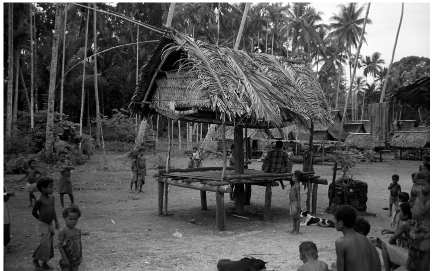
Fig. K2: Right frontal view of the bomiyoyeva . Note the large single central post ( kokola bwala ) which supports the horizontal canoe-shaped beam ( waga ) on which the entire loft ( tatom ) consisting of the roof ( katua ) and the floor ( bomakau ) rests.
