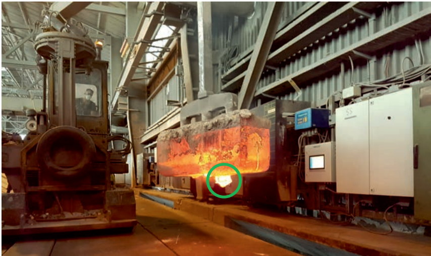
Fig. 1: Spike under anode marked with green circle.
