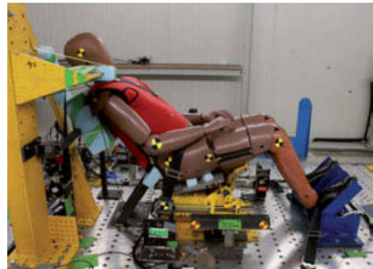
Fig. 7: Sled test setup with THOR-M 50 in reclined seating position (Thorax angle: 48°) – only to be used for validation of the vehicle environment in Virtual Testing.
