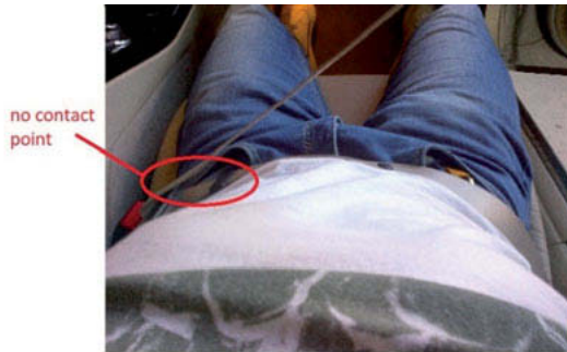
Fig. 9: The shoulder seat belt doesn't contact to the body with the fully reclined seatback in BMW 535i Touring (F11).
