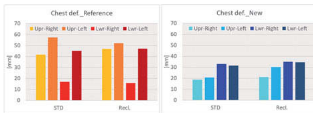
Fig. 14: Chest deflection results in Standard seat track position (Left: Reference system; Right: New system)
