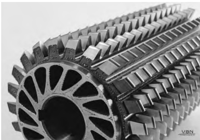
Fig. 1. Finished light weight gear cutting hob before coating. In the near hob end, the rest of additive manufactured support structure is seen (grinding not necessary). Material: Vibenite® 280 Optimum 70.
