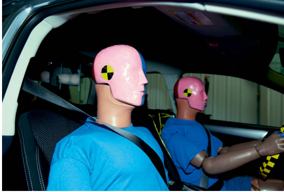
Abb. IV.3: Anthropomorphic Test Devices (ATD) aka crash test dummies Quelle: Wikipedia
